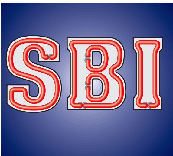
Illustration #5 Break the tubular look as a real neon tube installation would (A vs. B).
